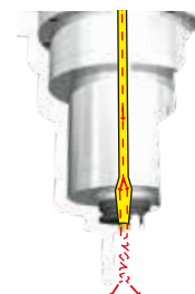
30 bar coolant through spindle
